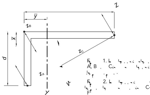
Surface area of members is included to help in evaluating how much paint or re-proofing (or any other material applied to the surface) will be needed. The shape perimeter of wide-angle sections has been calculated for two different cases as shown in Figure 3. Case A depicts a scenario where a concrete slab rests on top of the steel section, therefore, reducing the total steel section perimeter by a angle width. Case B depicts a full section perimeter without the angle width deduction.
