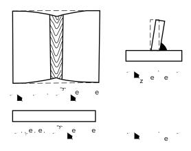
There are many factors that affect the distortion and shrinkage in a weldment, and distortion control principles go beyond simply reducing the weld size. Balancing the welds around the neutral axis of the member reduces the shrinkage moment and reduces the overall distortion in the member.
